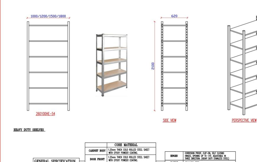
1.25mm THICK COLD ROLLED STEEL SHEET WITH EPOXY POWDER COATING.
